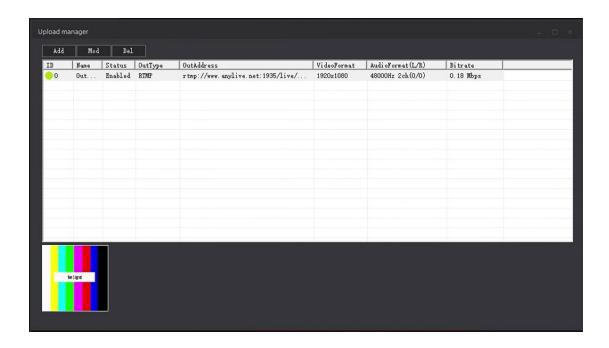
7 Double-click the enabled stream push address again, remove the check before enabling output, click OK, the stream push function is closed;
