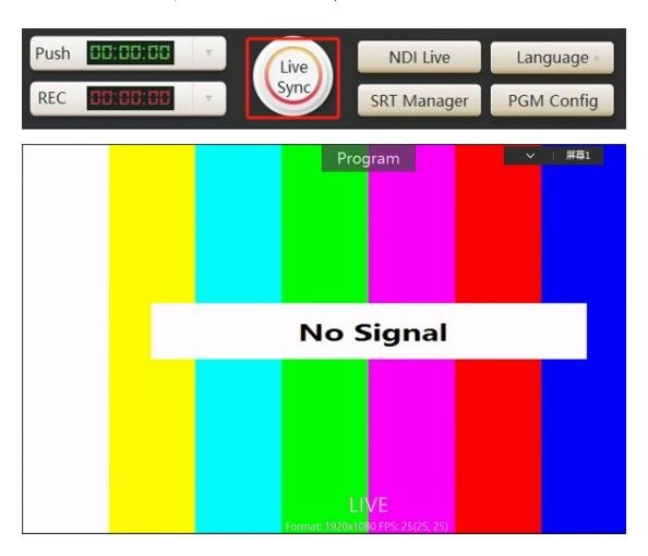
After the LIVE broadcast is enabled, the PGM window displays Live .
