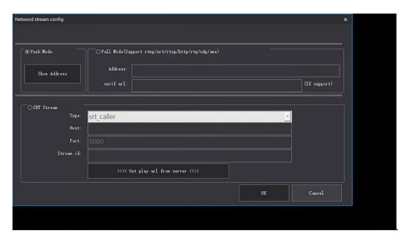
4 Push mode Click to view the push stream address, enter the address into a device with the same mode (in the same LAN), and the push stream will be displayed in the preview window.
