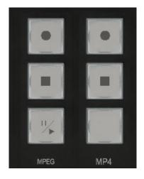
The first set of keys is the MPEG format recording, stop and live button, the indicator light is
