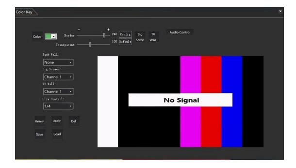
Click the photo picking button to enter the photo picking mode, as shown in the figure: (Note that the PVW pre-monitoring signal of the two-digit photo picking machine should be switched to the environment with green screen to perform the photo picking operation).
