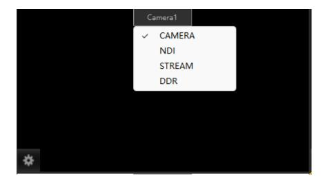
$(1)_{s}$  Camera: Camera signal source, which can be transmitted through SDI or HDMI;
