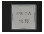
FAST/SLOW: Controls the rotation speed of the camera. When the indicator is on, the
