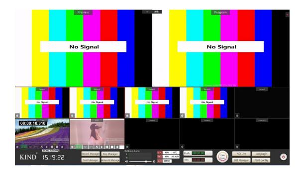
The main interface of the software is composed of PGM window, PVW window, 10-channel signal source pre-monitoring window, recording, live broadcast, push stream control panel and software mixer
