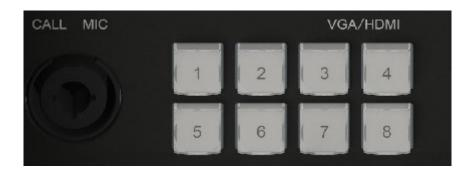
8 camera preset bits, use this button to quickly adjust the camera Angle
