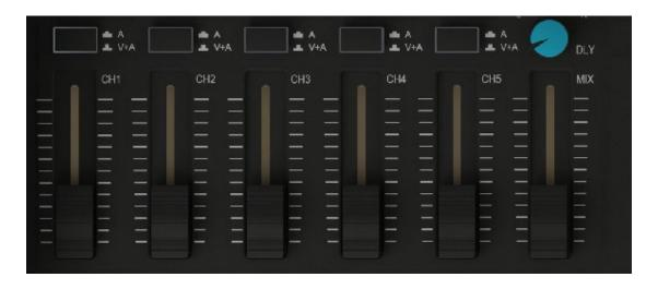
1 to 5 channel audio gain adjustment, corresponding to the backplane 1-5 audio source
