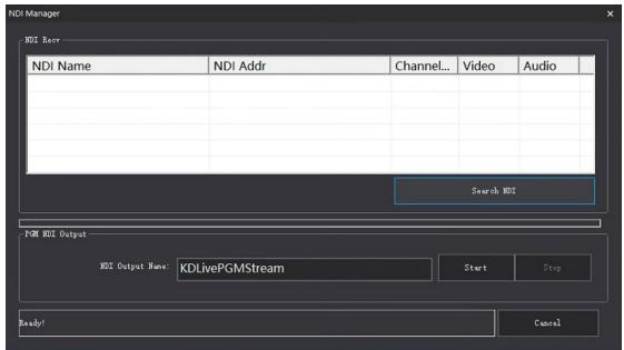
After the device is selected, the source Channel will pop up and Live Channel 1 will select the channel used. Cam serial number is the camera control address. The push, pull, roll, pitch and other movements of the NDI camera can be controlled through the camera address button.
