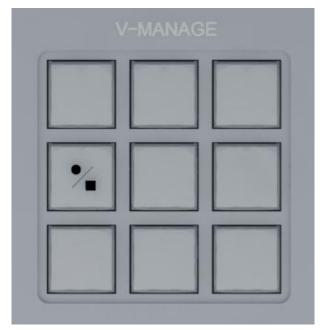
Recording button: If the indicator is not identified to the USB flash drive, the indicator is steady on. If the indicator is identified to the USB flash drive, the indicator is off. During recording, the indicator is blinking.
