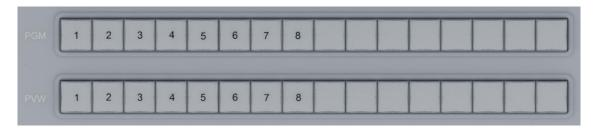
Main output screen and preview output screen source key, PGM row key as the main output key, that is, the live output screen. The playback channel will be displayed in the PGM screen, and the PVW row key will be the preview output screen, which will be displayed in the preview window.
