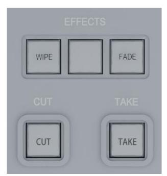
WIPE: Switch to enable transfer mode with the WIPE key set
