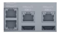
HDBoseT1 to 4 video input ports: supports signal specifications 3840×2160P25. 4K video source input (HD products support signal specifications 1920×1080P50 video source input)Hdmi 3/4 video input interface (HDBoset 3/4 for the same channel cannot input video source at the same time)
