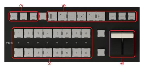
Transition effect key: includes stroke, fade in and fade out, picture in picture, video transition effect ®Image transfer effect type selection, multi-mode transfer effect, each key is a switching mode, each key has 4 switching modes, each press, the way to switch the screen is different; ①T-pusher: For quick switching between PGM and PVW;
