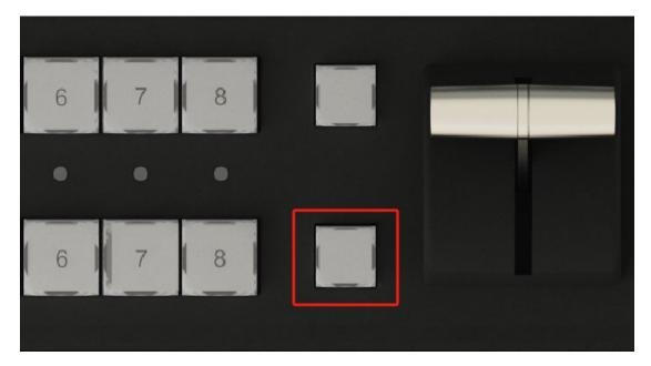
158 pre-monitoring mode switch key, press this button once PVW window generates 8 small pre-monitoring Windows (only 800H can achieve its function);
