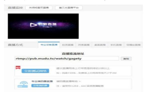
Configure RTMP live broadcast parameters, click the "RTMP Configuration" button, copy the push address provided by the live broadcast platform and fill in the "push point". If there is no user name and password, you can leave it out. Click save and quickly reset the encoder to start the push work.
