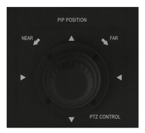
① Controller: can pass the camera orientation and focal length; The method of controlling the orientation of the camera, by controlling the up and down left and right rotation and left and right rotation of the rocker, the camera is pushed and pulled.
