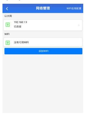
By adding the WIFI button on this interface, you can set the default WIFI network that the all-in-one is connected to  $\!\circ\!$
