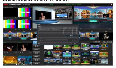
Double-click the searched signal source, double-click the designated channel 1 to 4 as the signal source, and then switch to select the following figure
