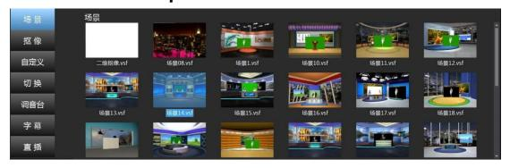
The thumbnail display of the scene above can be used to select different types of scenes according to the graphics. (When the scene is selected with the wheel encoder and the wheel encoder button is applied, the knob encoder of the device console can be used to perform the no-key operation on the scene application. The knob encoder can be rotated left and right to select between scenes. The knob encoder button is the application scene, click the knob encoder to return to the previous operation)
