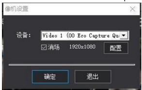
Set the capture card path in the device drop-down box to match the window number (for example, the IN1 window is set to Video 1)
